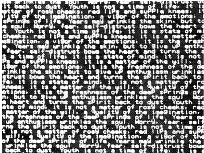
Figure 9 Photograph of 307,200 pixels on phosphor screen in size on 1 cm 2
